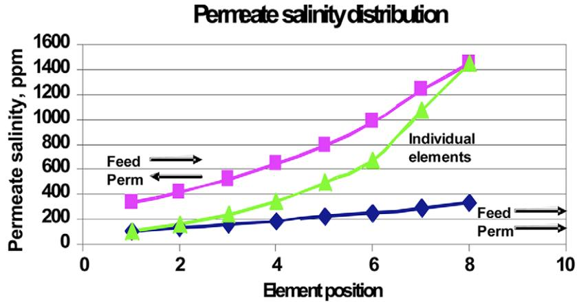
FIG. 17.3 Cumulative conductivity profile in pressure vessel as a function of relative flow directions.
