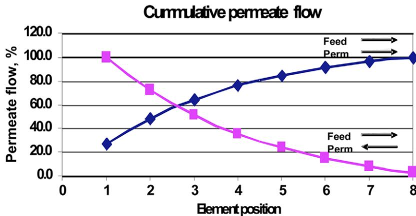
FIG. 17.2 Cumulative permeate flow in pressure vessel as a function of relative flow directions.
