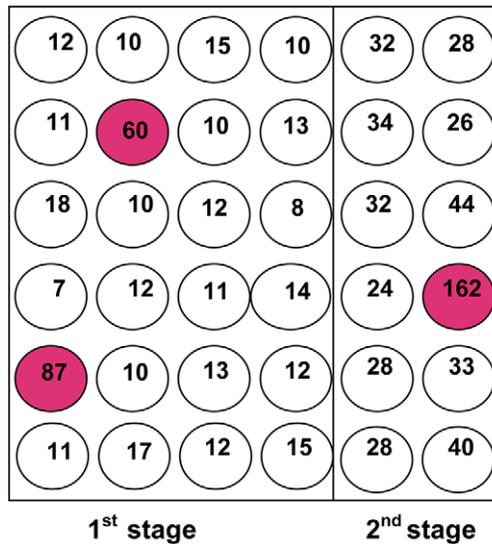
FIG. 17.1 Example of permeate conductivity measurement in a two stage membrane unit.
