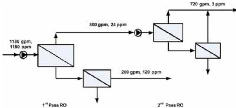
FIG. 13.16 Configuration of two pass system with processing of low salinity permeate (1st stage) from the 1st pass RO unit.
