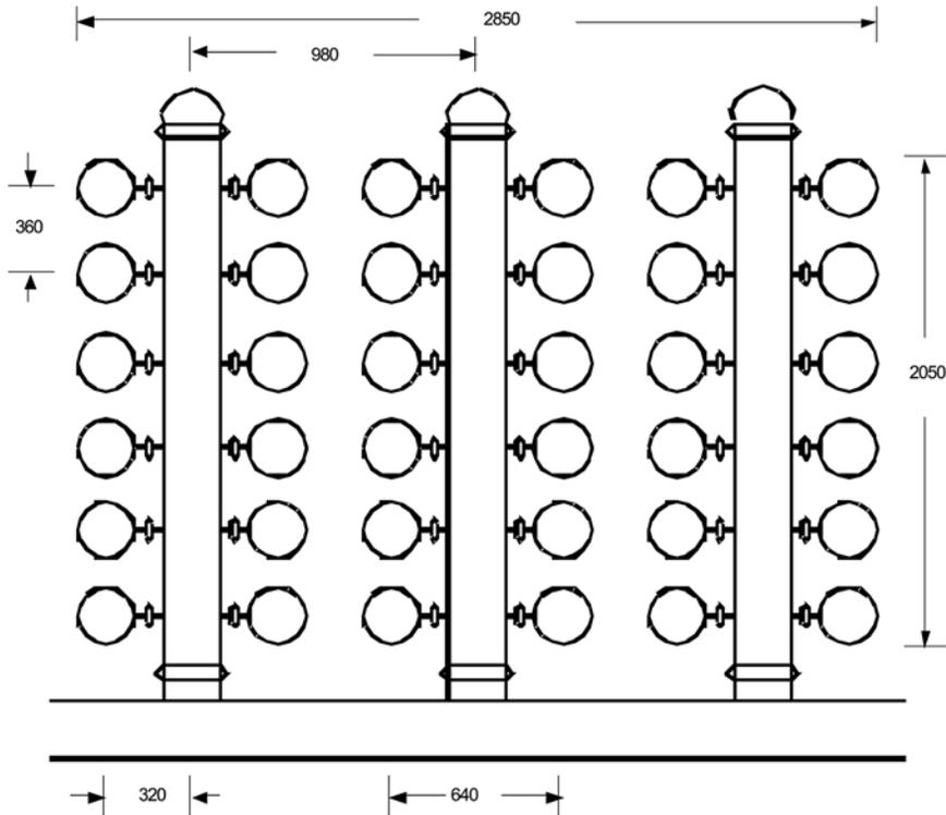
FIG. 13.2 Diagram of a membrane unit with sideport pressure vessels connected to the distribution manifold (measures in mm).
