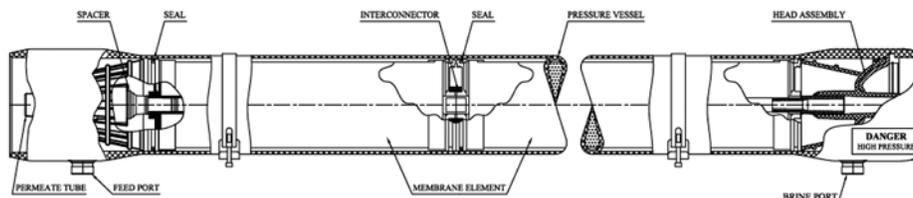
FIG. 13.1 Configuration of sideport pressure vessel with membrane elements (courtesy of Bell Industries).
