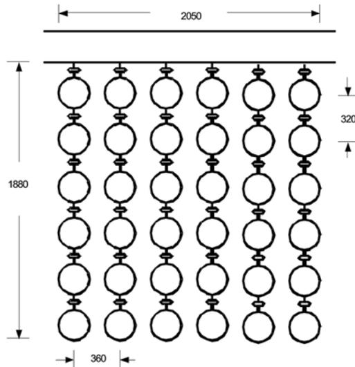
FIG. 13.4 Diagram of a membrane unit with multipoint pressure vessels connected to the distribution manifold (measures in mm).
