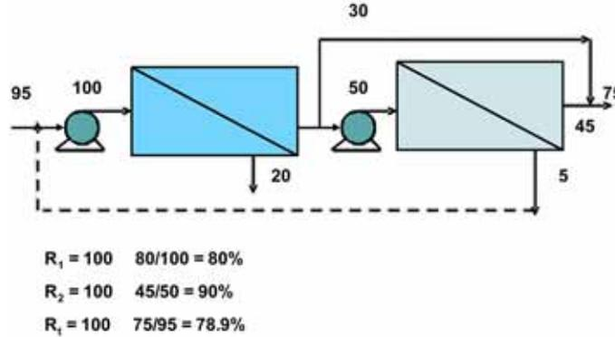
FIG. 13.14 Recovery rate in a partial two pass unit.
