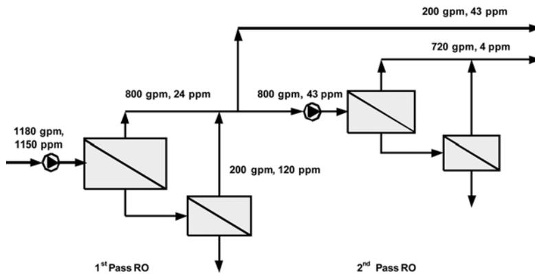
FIG. 13.15 Configuration of two pass system with processing of combined permeate from the 1st pass RO unit.
