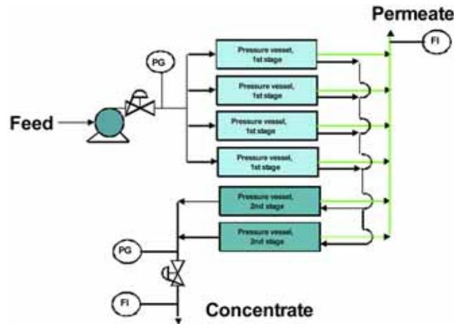
FIG. 13.9 Configuration of two stage RO unit.
