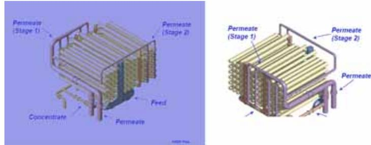
FIG. 13.10 3-D drawing of an RO train in a two stage configuration (courtesy CH2MHill).
