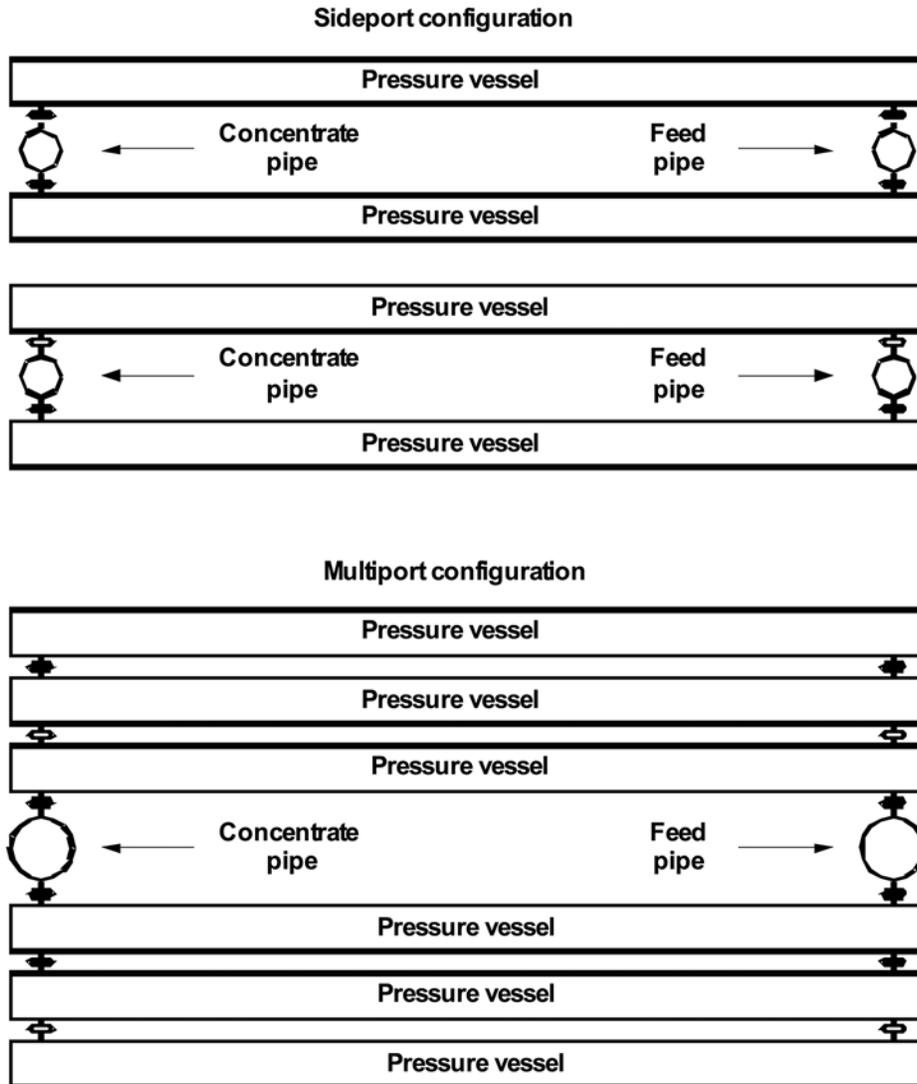
FIG. 13.7 Schematic configuration of a top view of sideport and multiport pressure vessel connections.
