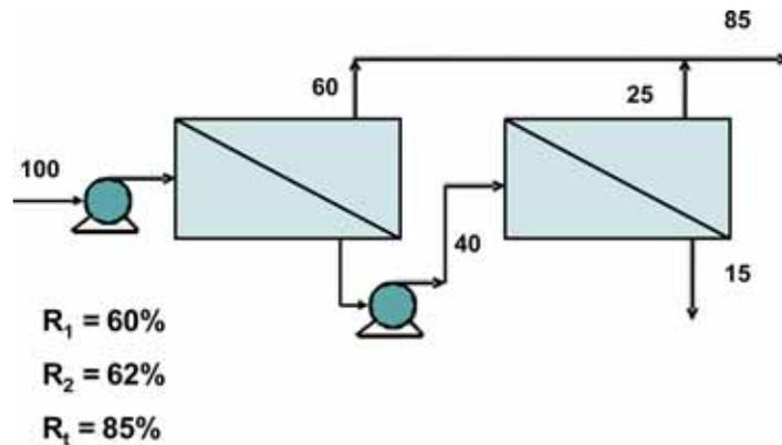
FIG. 13.11 Configuration of a two stage membrane unit with interstage booster pump.
