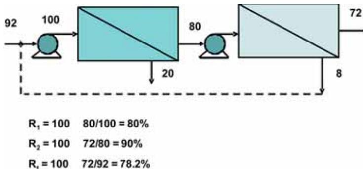
FIG. 13.13 Recovery rate in a two pass unit.
