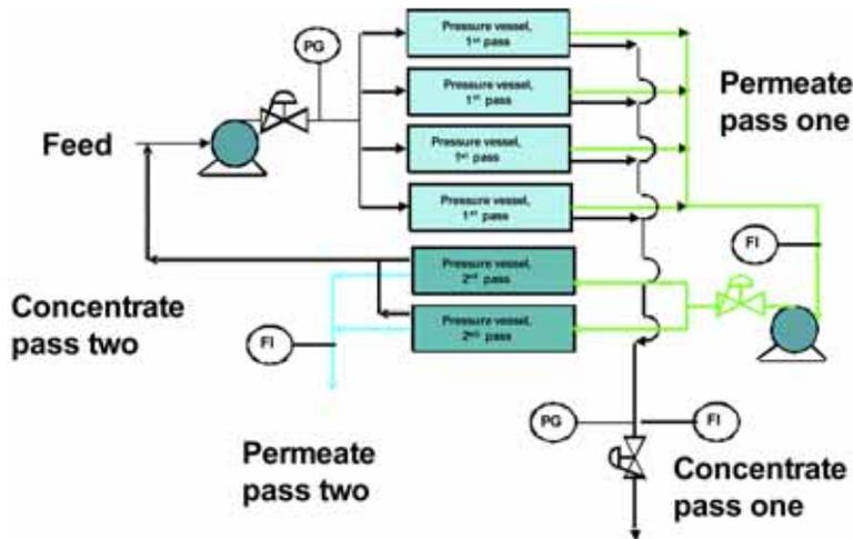
FIG. 13.12 Configuration of a two pass RO unit.
