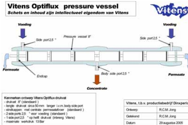
FIG. 13.8 Schematic configuration of Optiflux pressure vessel and corresponding flow path (courtesy Vitens).
