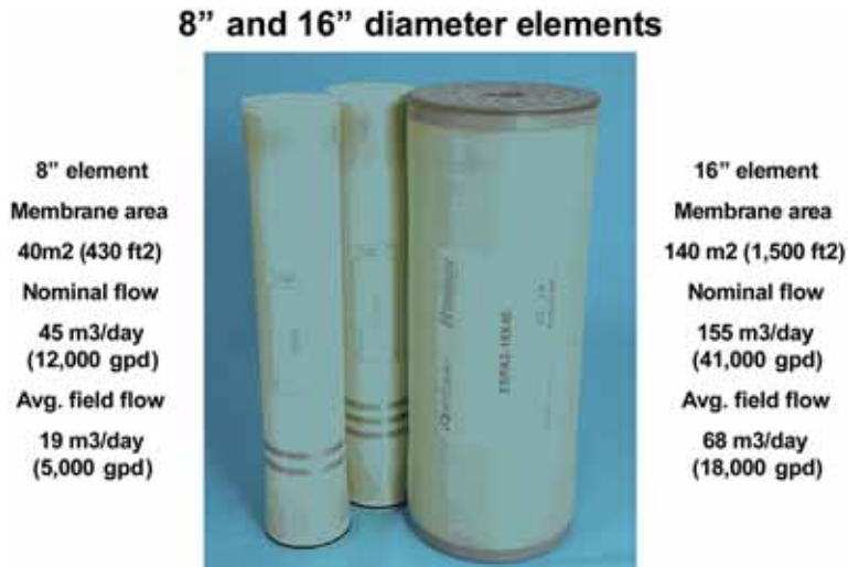
FIG. 12.16 Spiral wound 1000 mm (40") long 200 mm and 406 mm (8" and 16") diameter elements.
